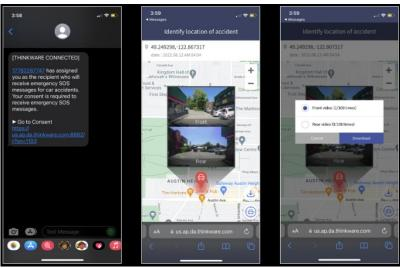
An emergency message can be sent to all registered contacts when the driver presses the REC button located on the dash cam for more than 3 seconds to request for help. In this situation, a 10-second video (5 seconds before and after the incident) will be uploaded to the server automatically. You can register the contact details of your friends, family, or associates and ensure that help will be on the way in case something happens.
