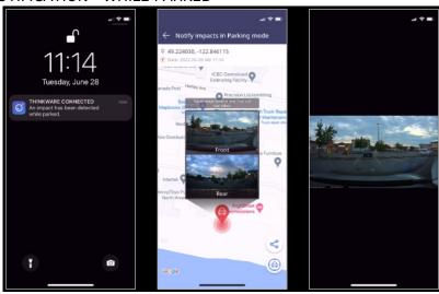
If an impact is detected while the car is parked, the app will receive a notification automatically. A 20-second video of the incident (10 seconds before and after the incident) is also saved on the Thinkware CONNECTED server if the user gives consent, and can be checked later from the app.
