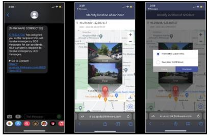
An emergency message can be sent to all registered contacts when the driver presses the REC button located on the dash cam for more than 3 seconds to request for help. In this situation, a 10-second video (5 seconds before and after the incident) will be uploaded to the server automatically. You can register the contact details of your friends, family, or associates and ensure that help will be on the way in case something happens.
