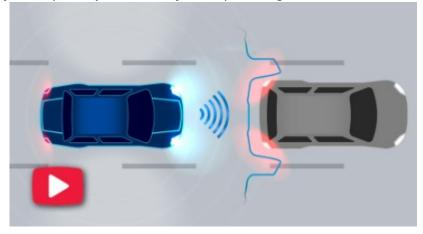
HIGH SPEED / URBAN FORWARD COLLISION WARNING SYSTEM (FCWS/ uFCWS) Accidents can be avoided by maintaining a safe following distance. Road Safety Warning System in the THINKWARE DASH CAM calculates the real-time distance between your vehicle and the vehicle in front of you, while driving above 30 km/h in expressways or under 30 km/h in a busy city, and issues a 3level early warning to the driver depending on the danger of collision.
