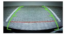
The camera shows static picture lines. These are guides to which the distance of the object can be determined where you drive your car to. Ideal for parking.
