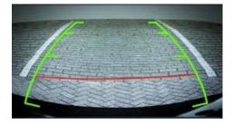
The camera shows static picture lines. These are guides to which the distance of the object can be determined where you drive your car to. Ideal for parking.
